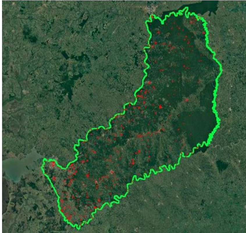
Figure 32: Spatial distribution of manually digitized samples through photointerpretation of Landsat images and the analysis of Normalized Difference Vegetation Index (NDVI) temporal signatures. In total, 1,268 polygons corresponding to nine land use and land cover classes were digitized.
